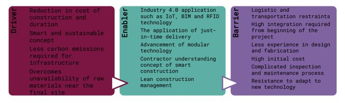
Figure 2: Drivers, enablers and barriers of modular construction
