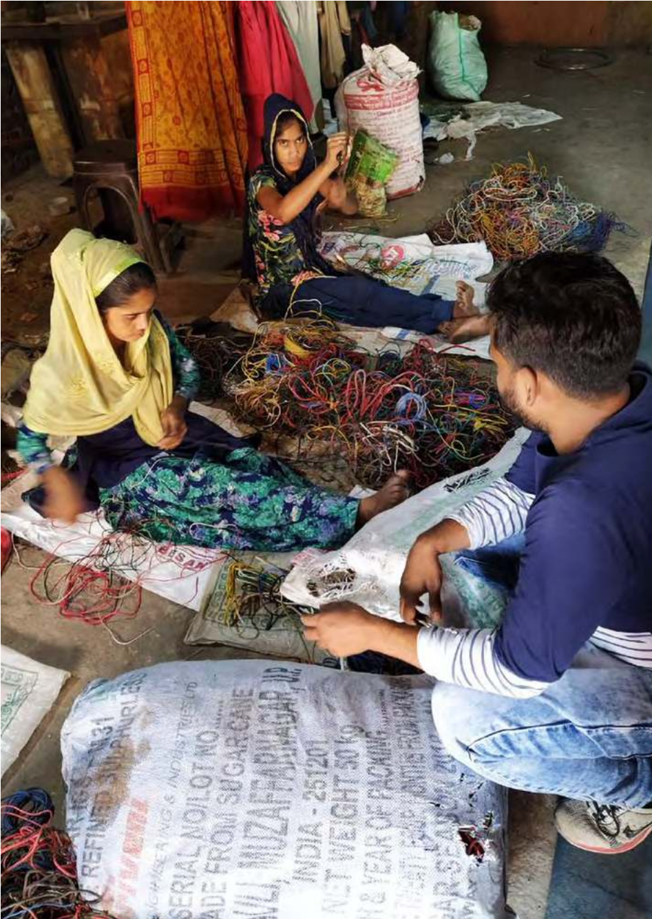
© E[co]work | Two women in Delhi stripping electric cables of their insulation.
